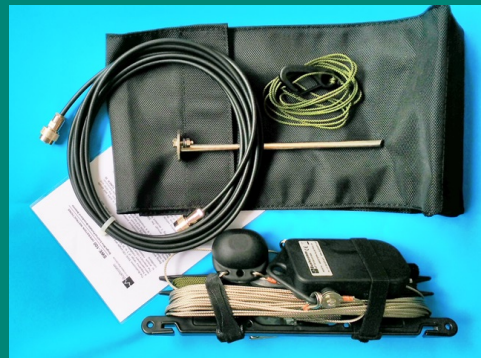
SWE-100P 24 metre Radiating element single wire end fed HF broadband antenna with quick deployment accessories.
