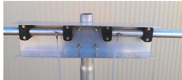
Leads showing the manner of attaching feed wires on the 5mm studs with wing nuts.
