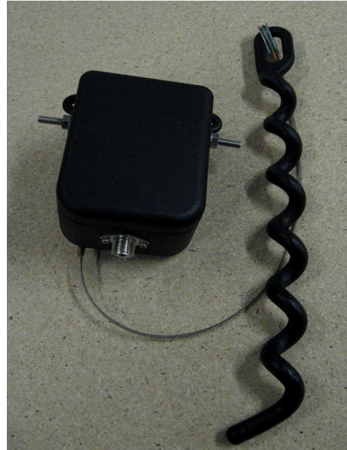
Above: Bushcomm Balun showing Pigtail strain relief ****
